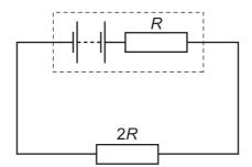
What is the ratio  $\frac{\text{power in external resistor}}{\text{power in internal resistance}}$ ?
