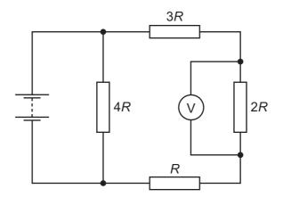
The voltmeter reading is 2 V.
